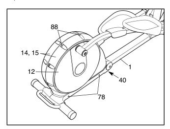
Adjust the position of the Side Shields (14, 15) until the Discs (12) no longer rub against them, and then tighten the Bolt Sets (88) and the M4 x 16mm Screws (78).
